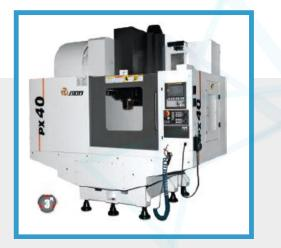
Purpose Precision cutting of parts using vertical spindles
