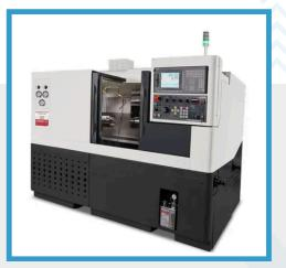
Purpose Precision cutting of parts into cylindrical shapes
