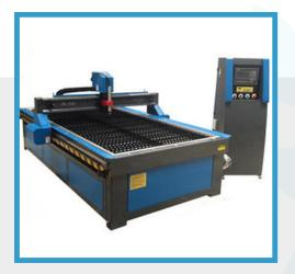
Purpose Cutting steel & stainless steel plates
